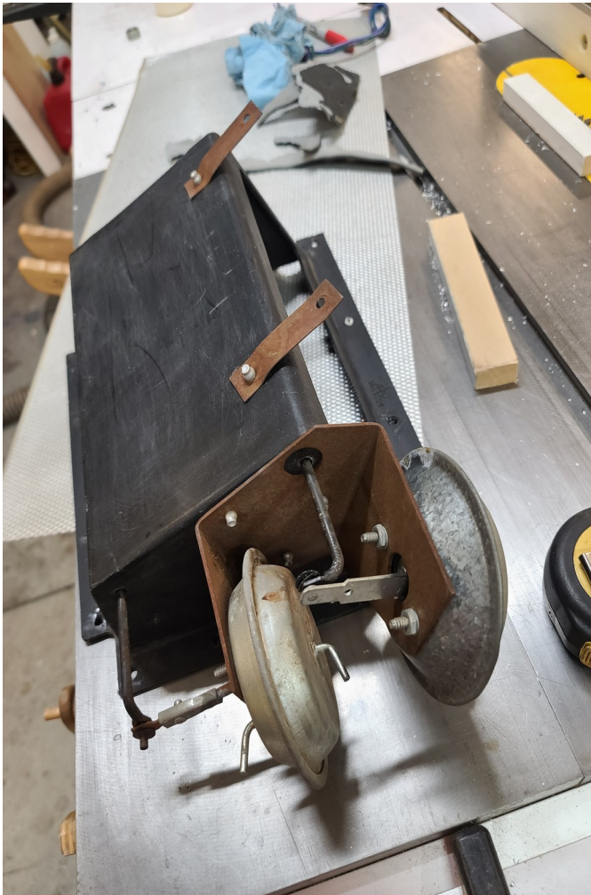
Rear part of air box. Left actuator is Heat, right one is Dash Air.
