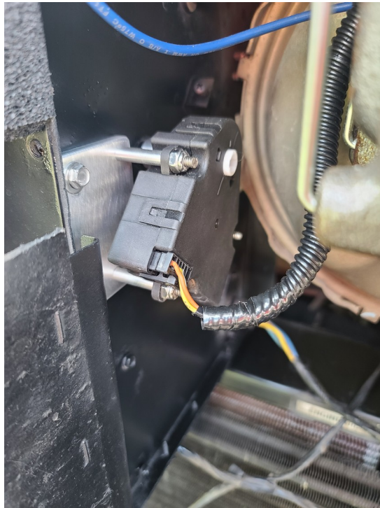
BDA as installed in the coach
