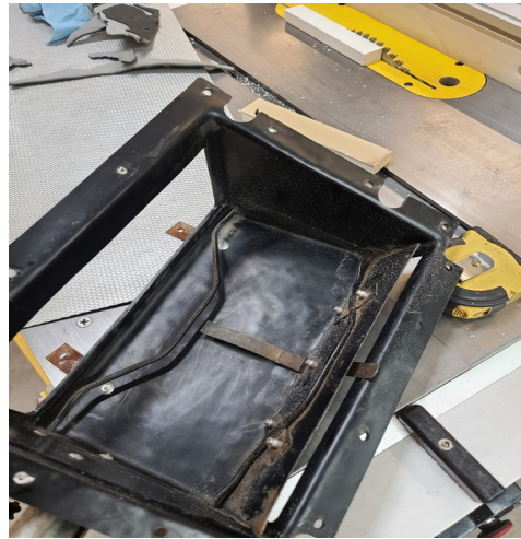
Original hinge rod with flap removed
