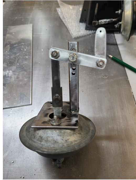
Modified defrost actuator with bell crank and stand welded on.
