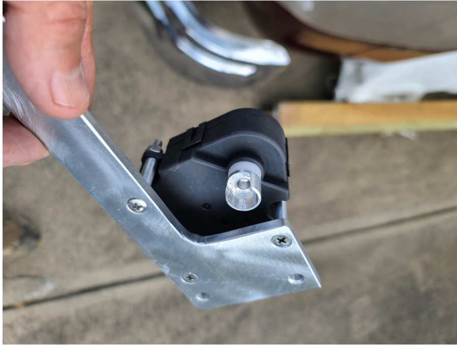
Blend Door Actuator from the Jeep mounted to the 1/4" aluminum mount bracket.
