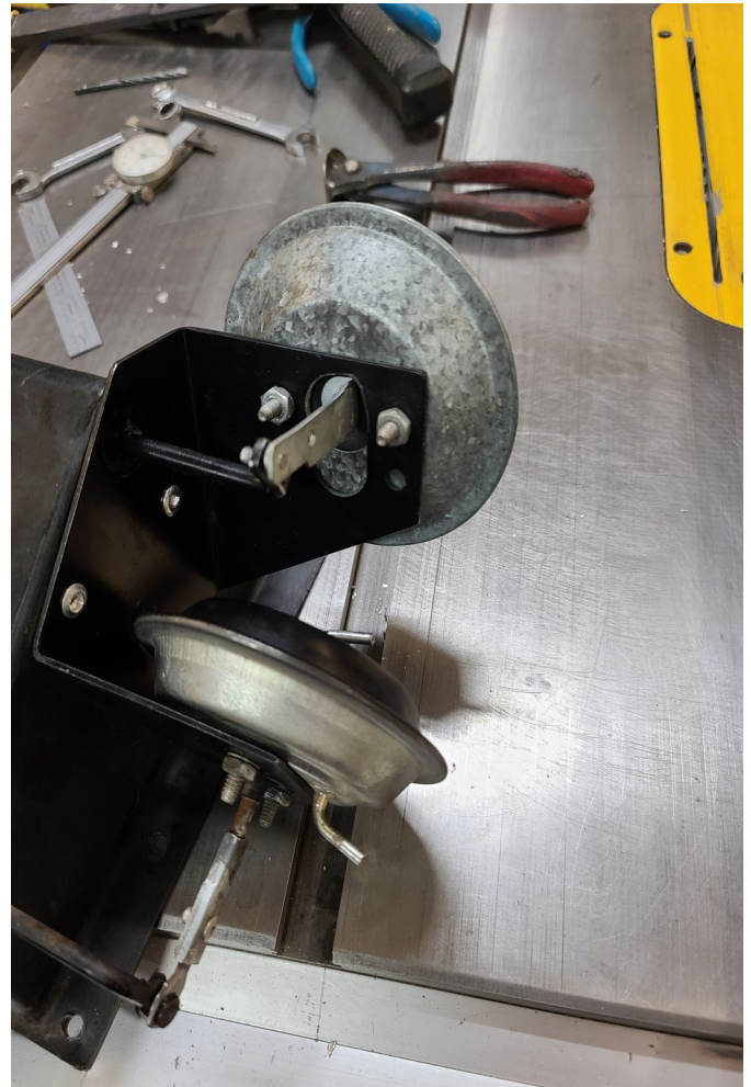
Modified. Notice bend in top hinge rod is reversed from left picture and position of actuator.
