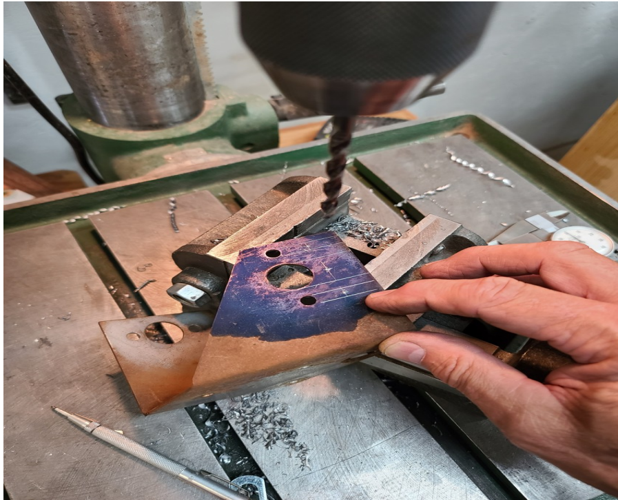
Elongating the Dash Air actuator pull rod hole, and drilling two new mount holes to reverse the action on the hinge rod
